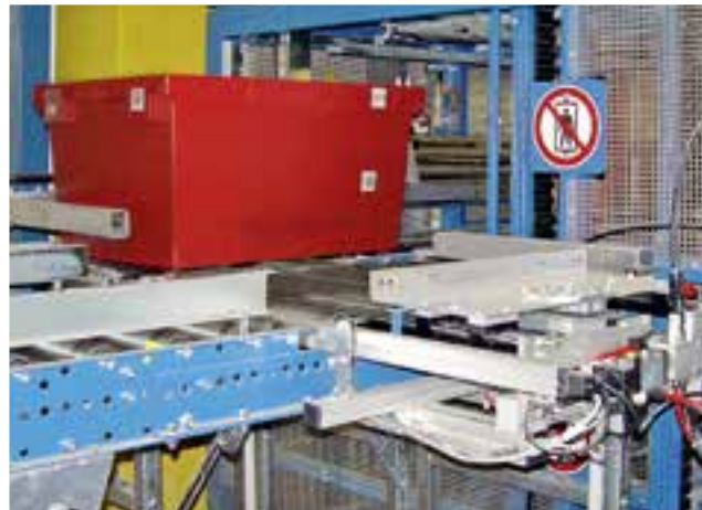
Feed station of an indexing conveyor for plastic boxes
