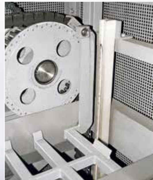
Driven wheel, plastic guide rail and platform of a circulating vertical conveyor for unit loads of varying dimensions.
