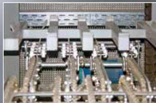
For unit loads of varying dimensions the platforms are designed in the form of a rake.
