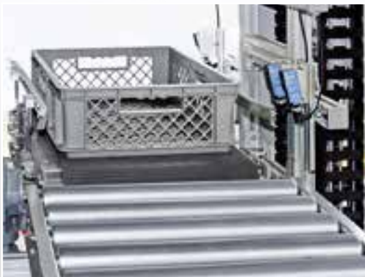
Transfer from belt conveyor on lifting carriage to the subsequent roller conveyor
