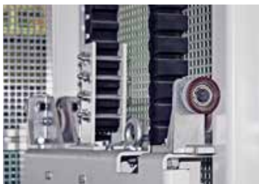
Vulkollan rollers guide the carriage
