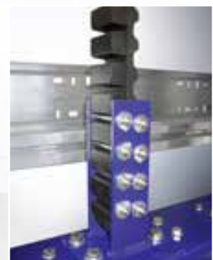
Rubber block chain fastened securely to the lifting carriage
