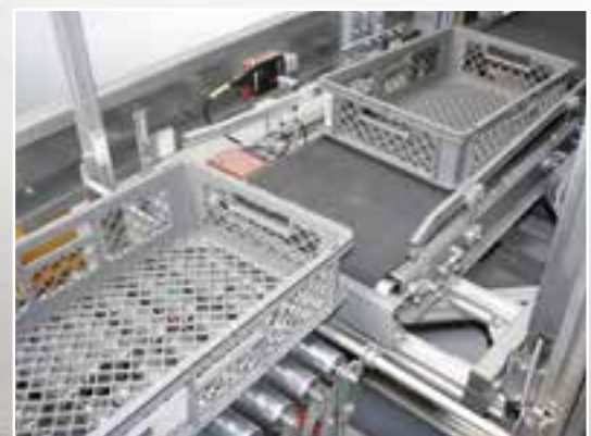
Feed station of a portal lifter with transfer onto the pivoting infeed conveyor, separating out the items.
